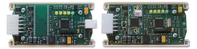
The device works with the feeding resistance range 8-36V. The consumption of the running device is 1.7W. In deactivated state the consumption almost equals 0after the signal 15 disconnection. Signal 15 is activated from approximately 1V level.
